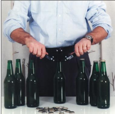
Put the crown cap onto the bottle, while keeping together the levers of the closing device, and then with ever increasing strength press them downwards. After a few rounds of capping you acquire more skill and speed in handling the device.
